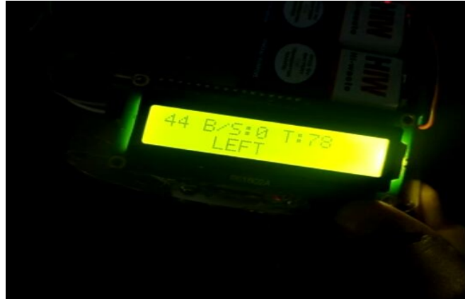
Fig. 8: Display showing wheelchair moving in LEFT direction
