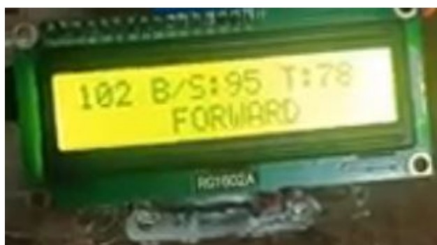
Fig. 5: MAX30100 sensor readings showing pulse rate as 102 bpm and oxygen concentration as 95%
