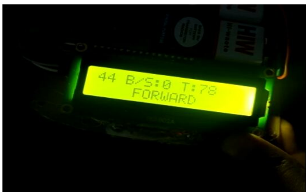
Fig. 6: Display showing wheelchair moving in FORWARD direction
