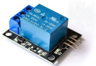
Fig.6. 5V power relay module
