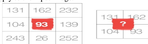
Figure 11.2: Left: The center pixel of a 3_3 kernel is located at coordinate (1;1) (highlighted in red). Right: What is the center coordinate of a kernel of size 2_2?
