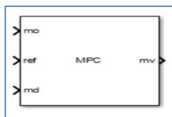
Fig. 7 MPC controller block
