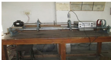
Fig: 1 Setup of Rotor system with crack disc
