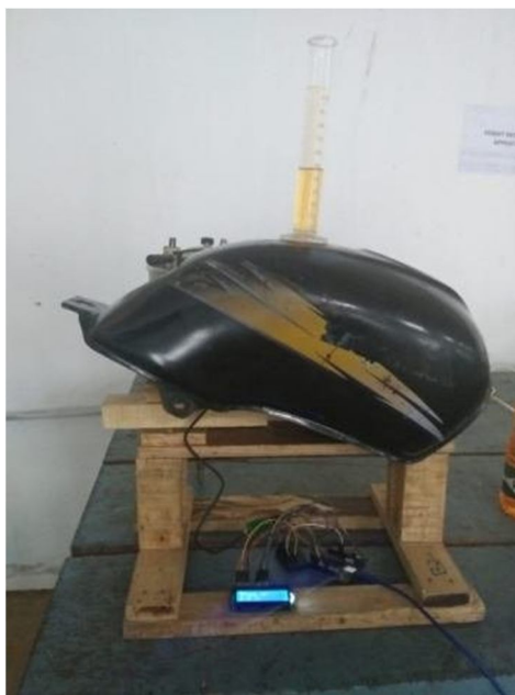
Fig. 2: - Load-cell sensor-based fuel measurement prototype for automobile fuel tank
