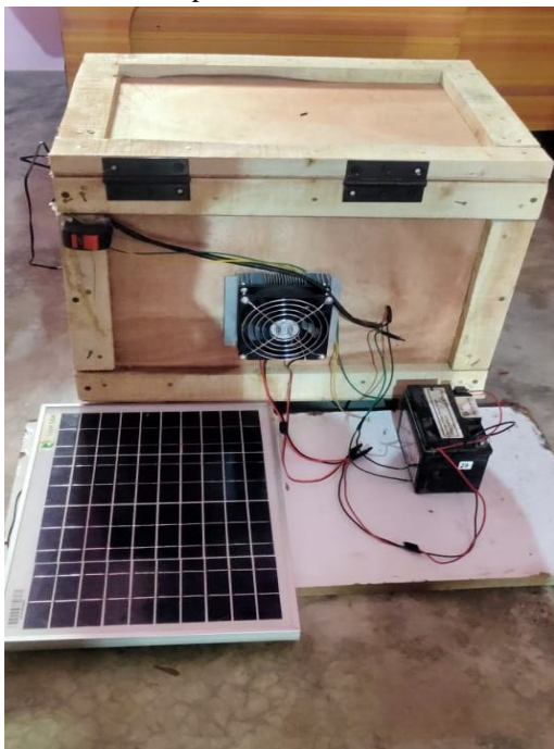
Fig -3: Experimental Setup where only polystyrene foam sheet is used inside the wooden box.
