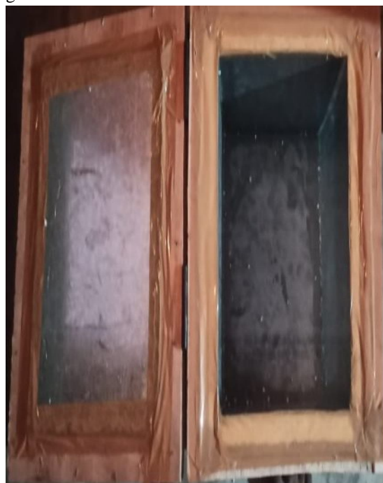
Fig -4: Top View of the Experimental Setup where GI sheet is attached with the polystyrene foam sheet.
