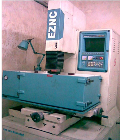
Fig1. Set up of Electrical Discharge Drilling on Sparkonix EZNC EMS-5535
