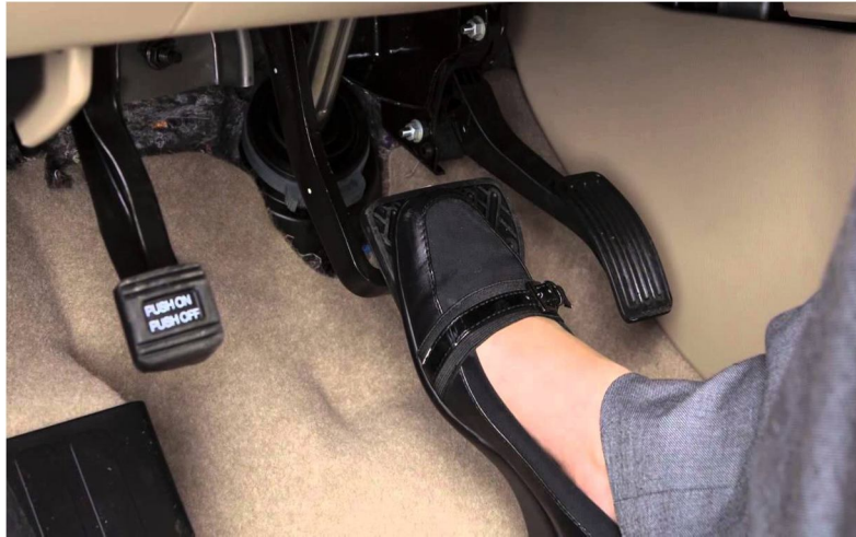
Fig.1.2.2.1. Service Brake or Foot Brakes
