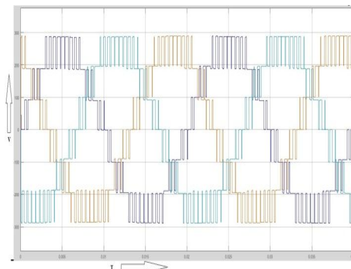
Fig. 6 Output voltage waveform for R-L load
