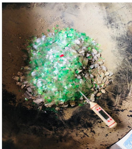
Fig 3 waste PET added to aggregates
