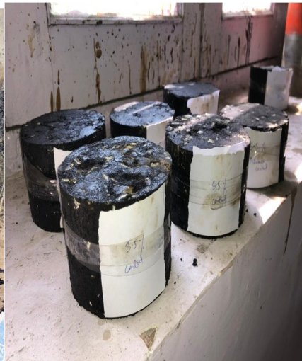
fig 4 samples with varying bitumen content
