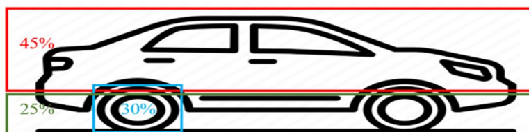
Figure 1: showing contribution of each part of a car for aerodynamic forces.
