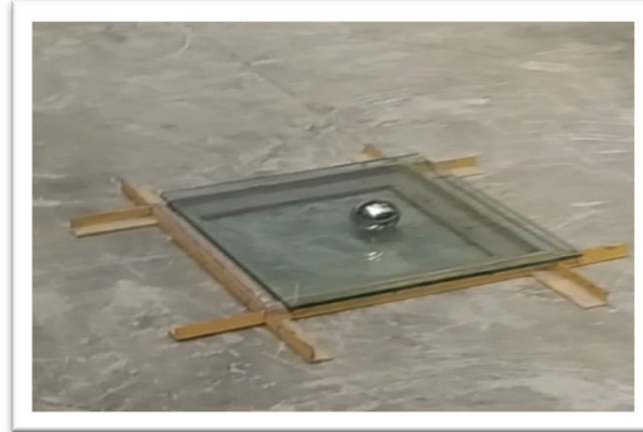
Fig.1: Ball Drop Test
