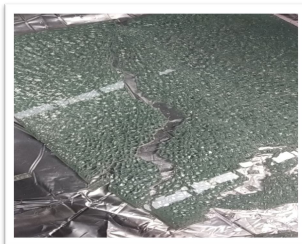
Fig.2: Fragmentation of Tempered Glass
