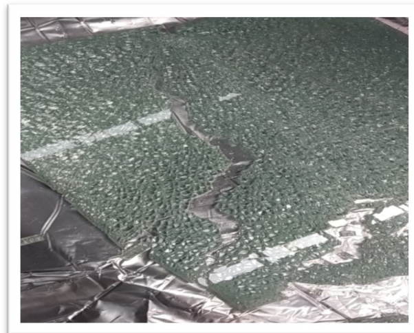
Fig.2: Fragmentation of Tempered Glass
