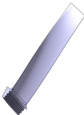
Fig. 5. Geometric model of turbine blade
