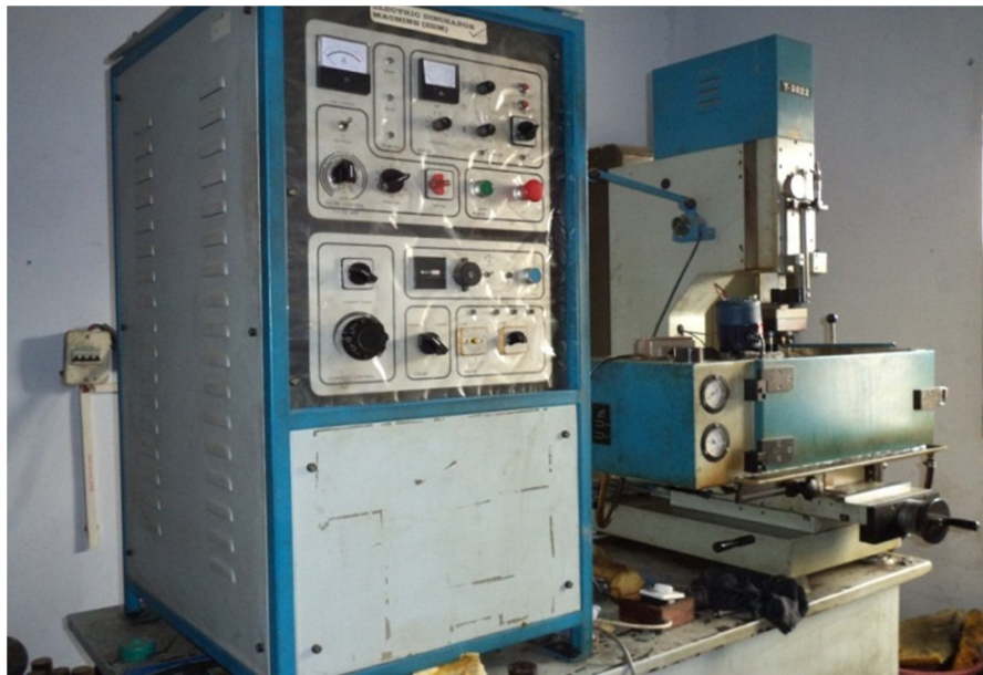
EDM machine with stirrer arrangement
