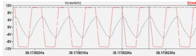
Fig.13 Output waveform of Relaxation oscillator with oscillating frequency f = 2 kHz
