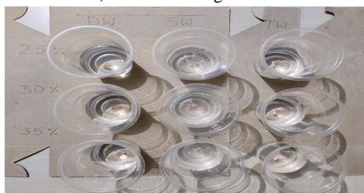
Figure 3: Composite specimens immersed in different water environment
