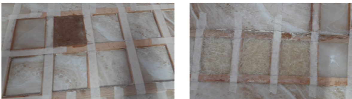
Figure 1: Fabrication of coir and sisal fibre reinforced composite
