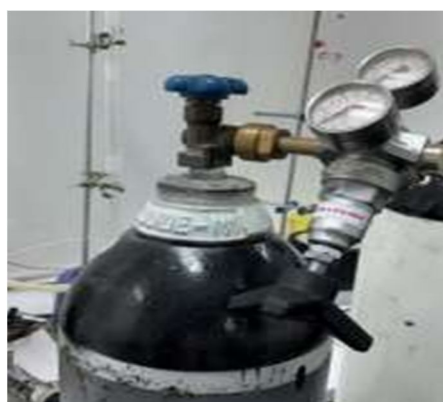
Air Supply Tank.
