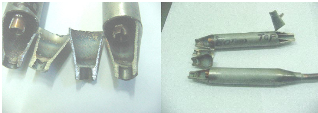
Fig. 6: Brazed Joint Cutted for Inspect for Penetration
