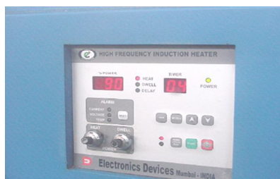
Fig. 4 Power Control Unit
