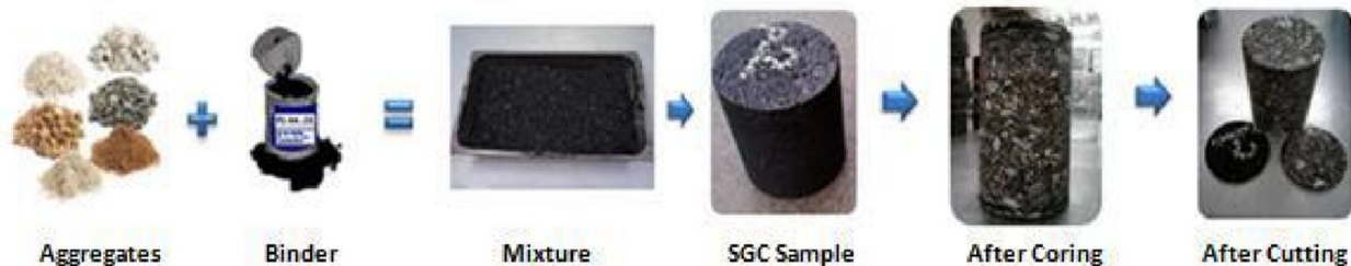
Figure 7: Diagram showing preparation of specimen for stress relaxation test
