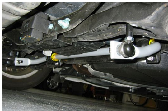
Fig No2: Fitment picture of ARB on vehicle
