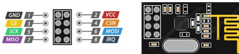
nRF24L01+ Pinout
