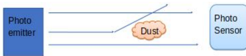
Fig. 3 Reflection, Refraction, and Deflection of light waves by Dust particles
