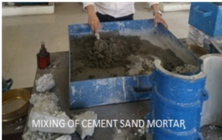
Figure 2 Mixing of cement sand mortar
