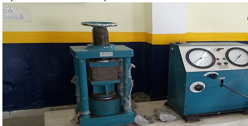
Figure 3 Compressive strength test on concrete
