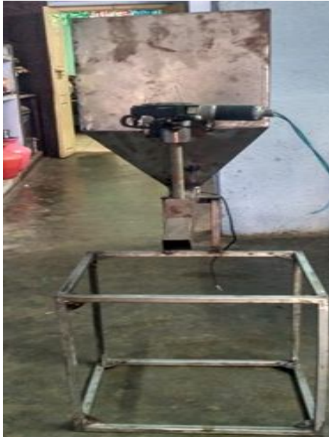
Fig 1: Fabrication of Smart Storage and Dispensing Machine for Food Grains Fig 2: Internal Components of the Machine
