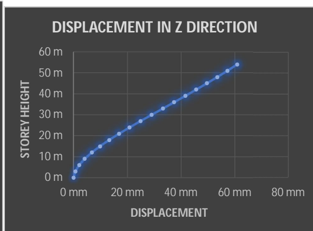
Figure 6b: Displacement in Z direction
