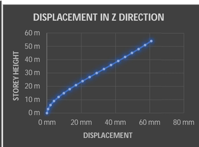
Figure 6b: Displacement in Z direction
