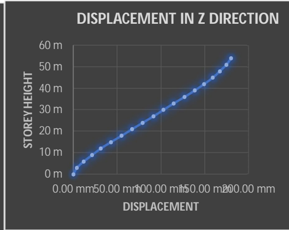
Figure 4b: Displacement in Z direction
