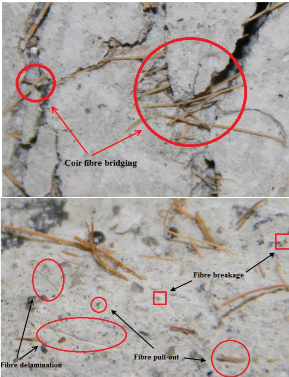
Figure 12: Bridging of coir fibres
