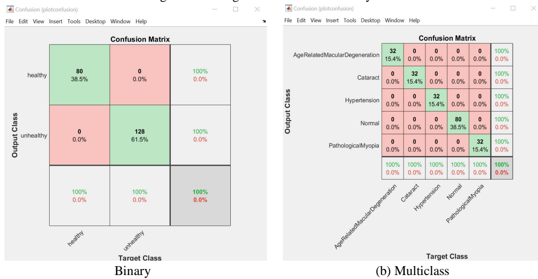
Fig 3. Confusion matrix of training dataset. (a) Confusion matrix of binary classification (b) Confusion matrix of category multiclass
