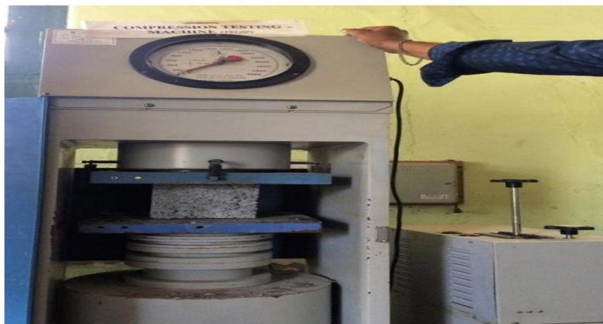
Figure-3.2 Compressive Testing Machine
