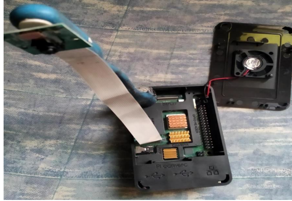
Fig.1. Connectivity of Camera with Raspberry Pi
