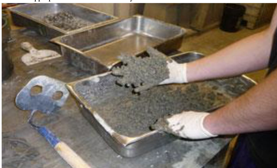
Fig showing mixing of concrete
