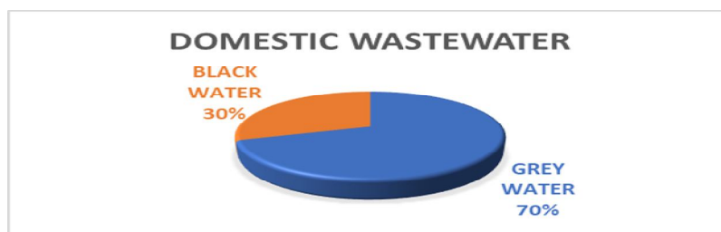
Fig. No. 01 – Composition of wastewater
