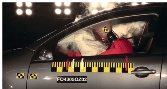
Fig. 1: Airbag deployment during crash
