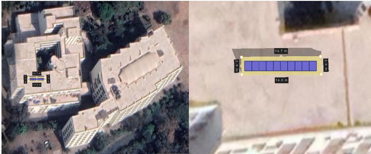
Fig. 5: a) Solar array placement at the site and b) Close-up of the solar array (Helioscope and google maps)
