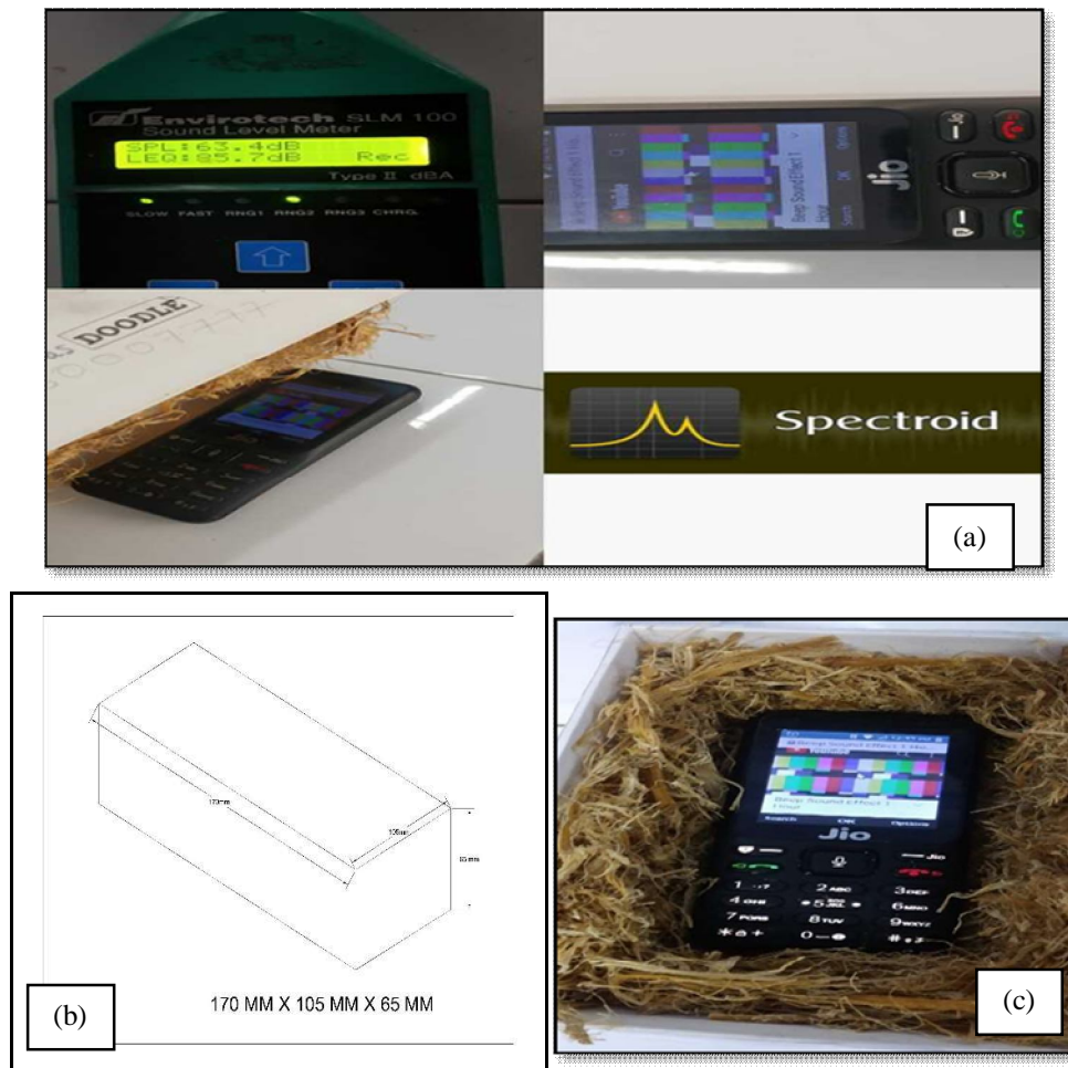
Fig. 13- Testing image- (a) equipment; (b) test box; (c) sound source inside the box
