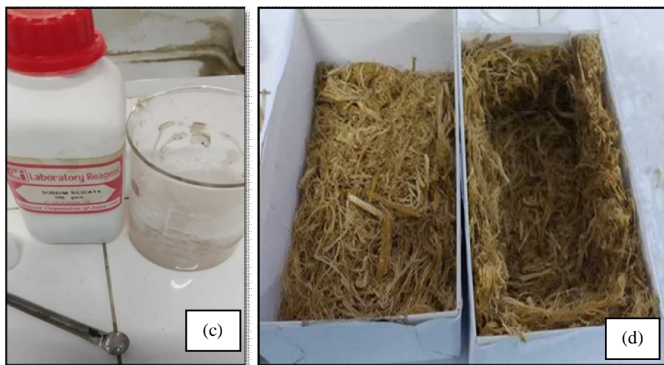
Fig. 12- Fabrication process stages- (a) moulded sheet; (b) cutting as per required size; (c) Adhesive preparation; (d) Lining in the test box
