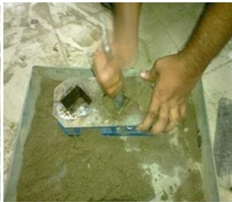
Tampering the layer with rod
