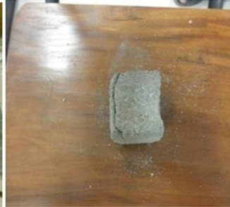
Cracks develop after crashing.
