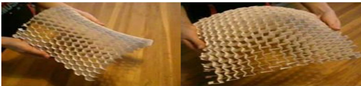
Figure 3. a) shape shown by non-auxetic materials, b) shape shown by auxetic materials[9]
