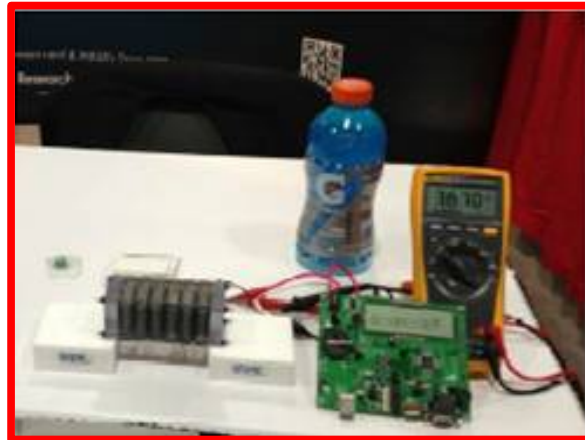
Fig(14)Microprocessor and LCD powered by bio battery
