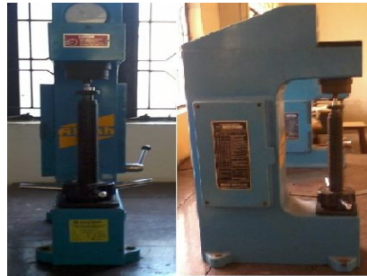
Fig 3.7: Brinell Hardness Testing equipment.
