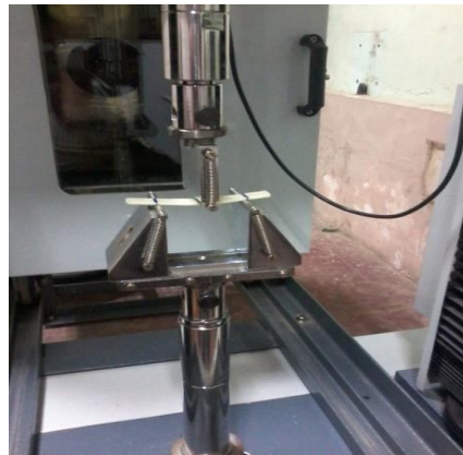
Figure 3: Loading arrangements for flexural test
