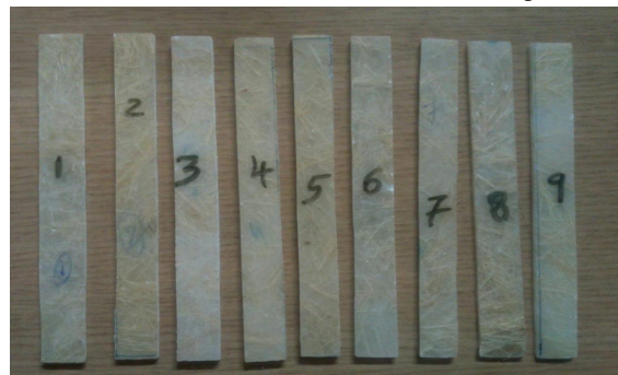
Figure 4: Flexural test specimen samples
