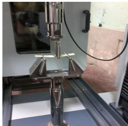
Figure 3: Loading arrangements for flexural test
