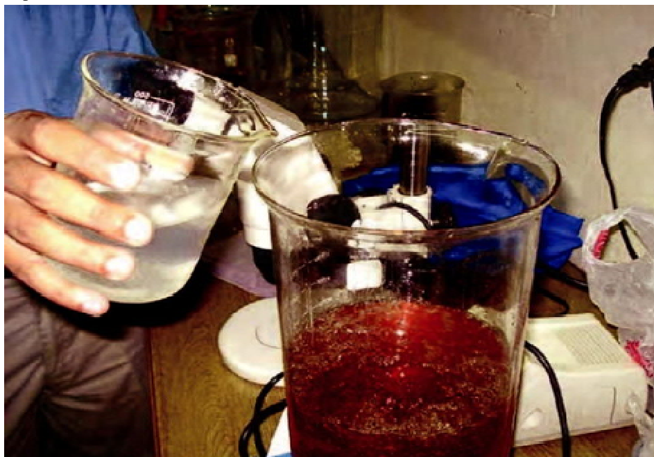
Fig. 2 Mixing the catalyst sodium hydroxide to methanol to liberate sodium methoxide
