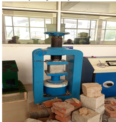
Figure 2: Compressive strength test using CTM
