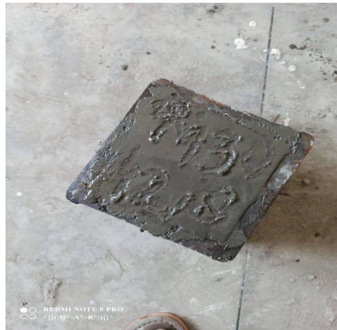
Figure 1: Casting of concrete cubes
