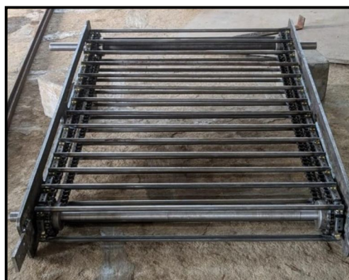
Fig. 6 Photo of the Actual Conveying system.
