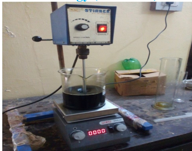
Fig.1 Experimental setup for biodiesel production
