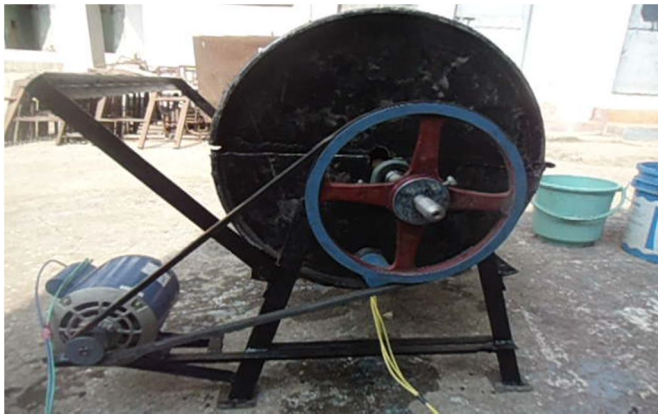
Fig 3: Side view of Cloth Dyeing Machine (Actual Photo)
