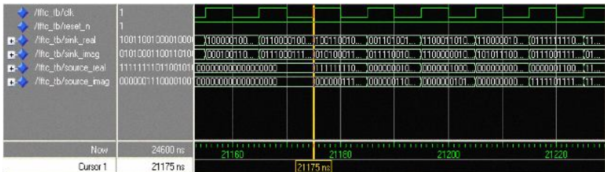
Fig:4.Simulated waveform of the 1024-point FFT
