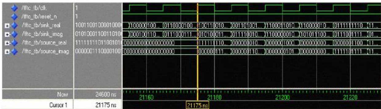
Fig:4.Simulated waveform of the 1024-point FFT
