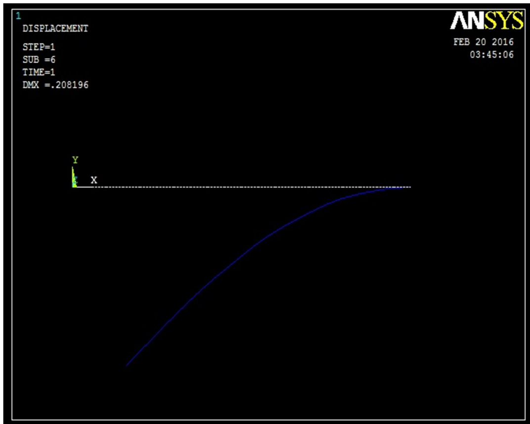
Figure 2: ANSYS deflection when 500gm weights applied
