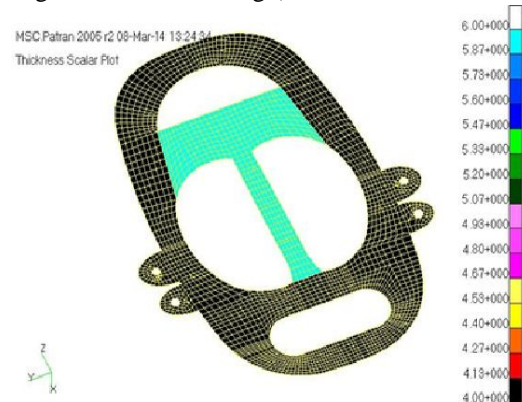
Fig 12: Bulkhead with 4mm and 6mm thickness
