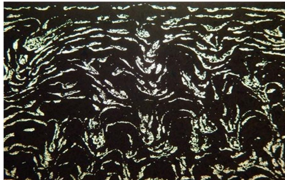
Transparent Concrete When Optical Fibres Are In Organic Distribution
