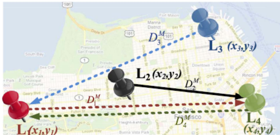
Fig. 2. PPFRVP scenario, where the fairness function is g = \text{argmin}_i (DM_i) . The dashed arrows represent the maximum distance DM_i from each user u_i to any user j \neq i , whereas the solid line is the minimum of all such maximum distances. The fair rendezvous location is L_{fair} = L_2 = (x_2, y_2) .
